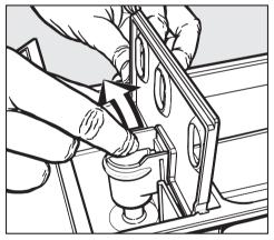
■ Remove the siphon tube from compartment <a href="#">\®</a>.
